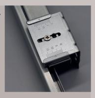
This built-in flexibility allows the single-extension, soft-close runners (with a 30kg weight rating) to be adjusted in precise 1mm increments using only a screwdriver, ensuring they clear the wardrobe door hinges seamlessly.
